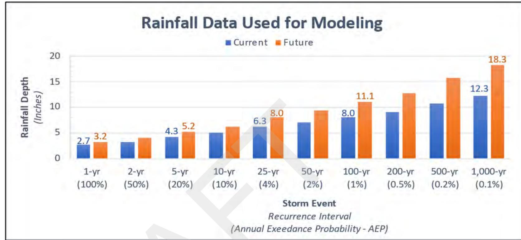
Graphic #8: NOAA Atlas 14 24-hour rainfall data used for modelling. “Current” depths use the median value of the Atlas 14 data set, common practice for determining current rainfall. “CCIPF” depths are the upper bound of data set (Atlas 14++), a simple methodology for determining climate change informed predicted future (CCIPF) rainfall. (Report Section 2.1)
