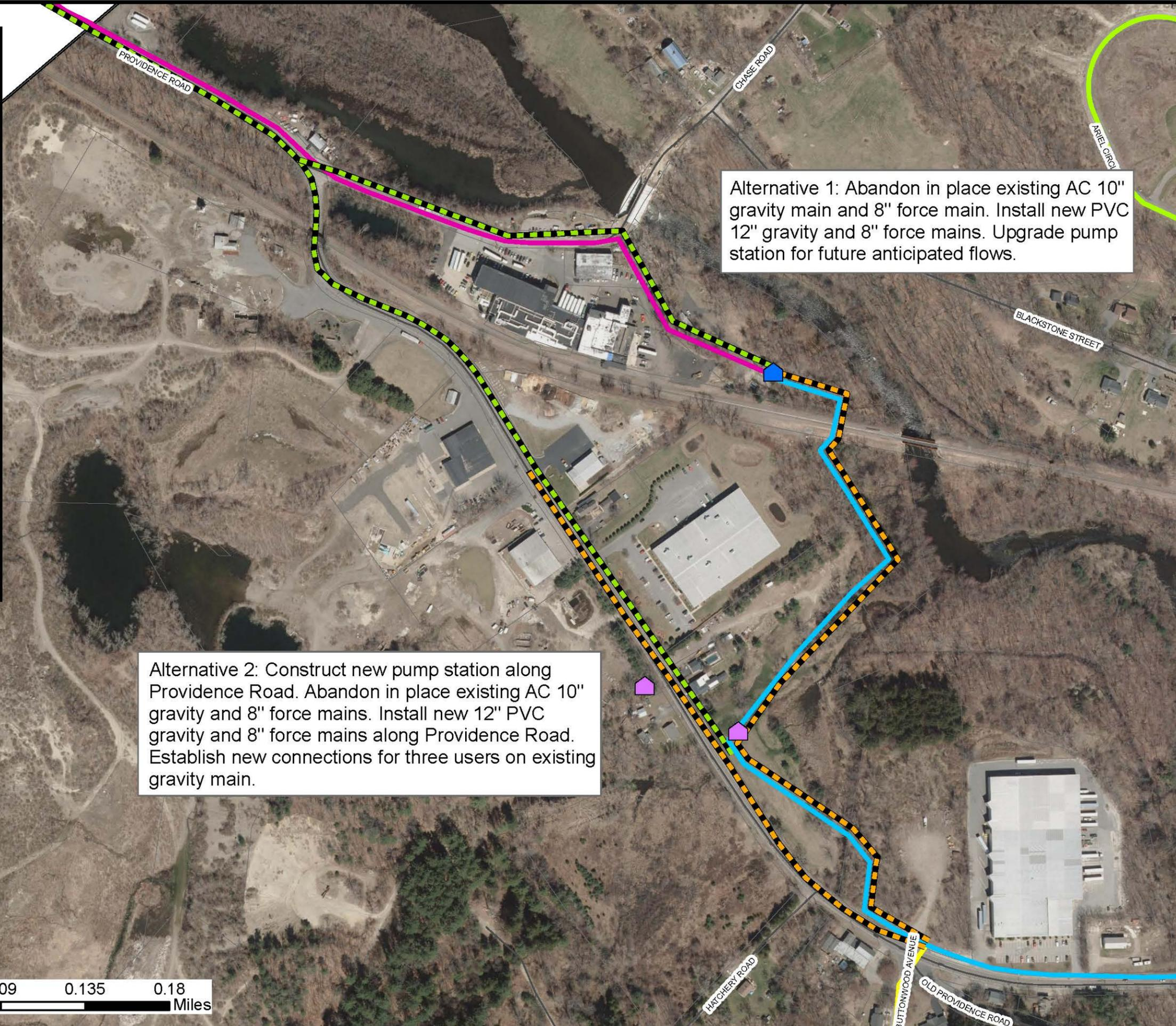
Alternative 1: Abandon in place existing AC 10" gravity main and 8" force main. Install new PVC 12" gravity and 8" force mains. Upgrade pump station for future anticipated flows.
